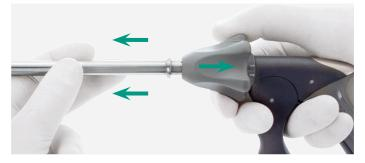
**3.** Hold instrument shaft. Pull back star wheel to the stop in the direction of the handle to disengage the safety ring and to release the instrument shaft. To remove safety ring from handle pull it off towards rear of handle.
