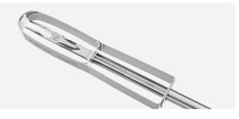
**5.** Pull push-rod out of inner tube.
