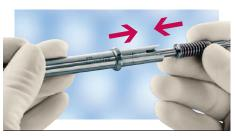
Insert inner tube and push rod into shaft.
