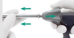
1 3. Hold instrument shaft. Pull back star wheel to the stop in the direction of the handle to disengage the safety ring and to release the instrument shaft. To remove safety ring from handle pull it off towards rear of handle.
